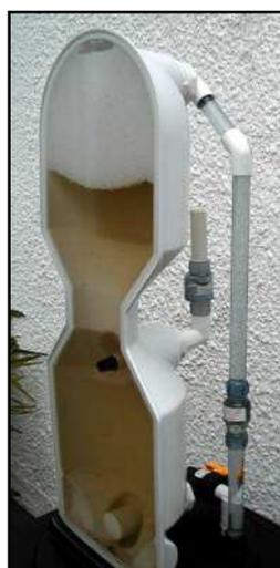
**Air inlet and outlet non-return valves clearly shown**
