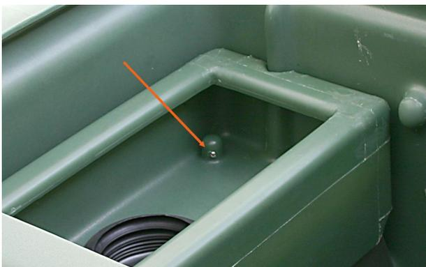
For closer access to the *internal pipework*, it is possible to remove the *floating weir* by removing the *retention screw(s)* (see picture) and pulling the *support rods* from the sockets in the underside of the *floating weir*.
