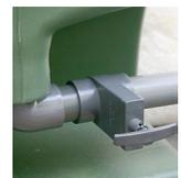
The valve can be opened and waste directed into a bucket. Alternatively the outlet of the valve can be extended to a sewer or remote sump capable of handling the volume and concentration of wastes. The waste pipe must be free draining and without an excessive number of bends, as the waste material is likely to include large amounts of solids.
