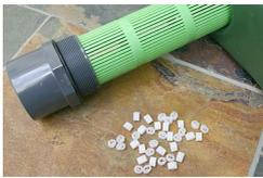
Unscrew the *outlet strainer* to check that the grade fitted is the one suited to your situation (See Note 1). Wrap the threads with PTFE tape to improve watertightness and ease future removal, and screw it back in taking care to avoid cross-threading. If the sealing ring is gently compressed this will give a further watertight seal. The outlet strainer may need to be removed for future maintenance, so ensure that any
